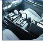
**30" Enclosed Console** Mount up to 17" of equipment and store your items in the 13" carpeted storage box. Comes complete with vehicle mounting brackets and filler plates to enclose top of console less internal options. **C-3011**
